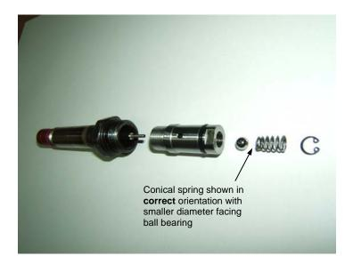
Exploded assembly of emergency manual lowering valve (VSMA)
